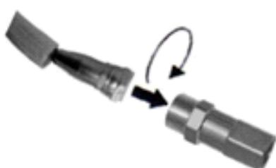
Remove the protective caps on the coupling halves and manually screw the matching female halves (on the refrigerant lines) onto the halves on the components or units.
